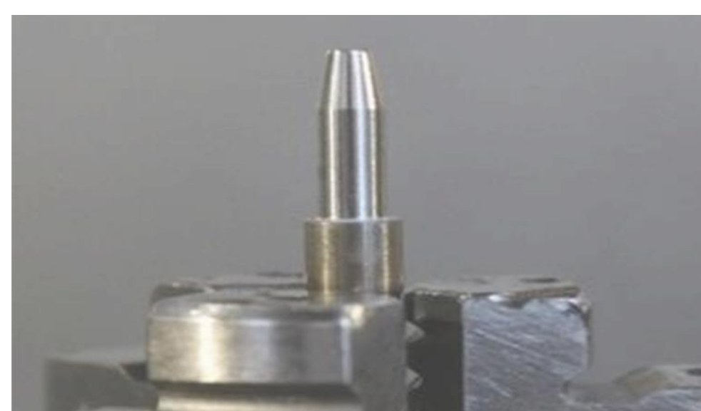
CNC manufacturing of conometric coupling
