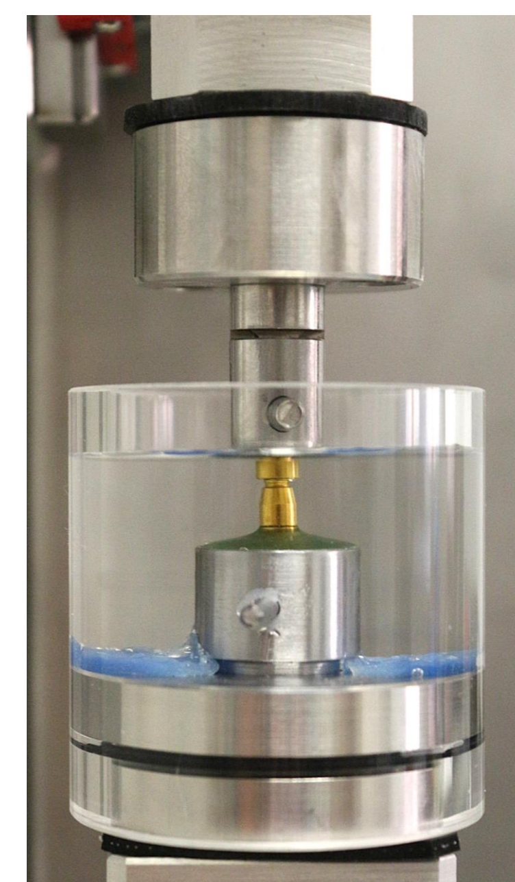
Tests performed with perfect passivation in artificial saliva.
