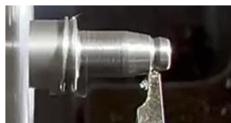
Manual turning of the retentive groove
