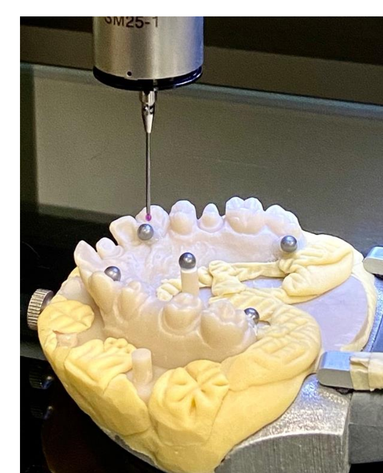
Zirconia model calibration with OCMM, SmartScope Flash CNC 300
